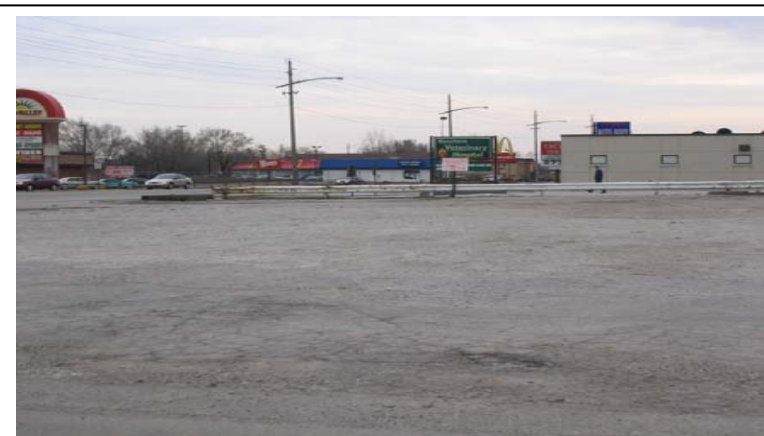
Paved, impervious surfaces such as this expansive parking lot contribute to storm water runoff and groundwater pollution. Incorporating landscaping and sharing parking areas can help.
